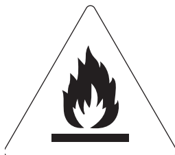
Caution:Risk of fire/ flammable materials
